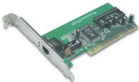
Figura 2.1 Tarjeta Ethernet
