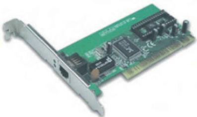
Figura 2.1: Tarjeta Ethernet.
