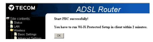
Or by pushing the physical push button placed in the rear panel in the router and labelled with the wireless symbol (HW method), at least during 8 seconds
