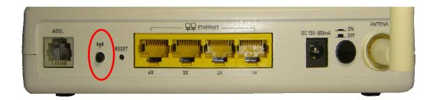
From this moment on, you must activate the WPS method in the client (for instance, a wireless USB adapter which supports this option), by pushing also its corresponding WPS push button, within a time window of 2 minutes as maximum. If you don't push the WPS client push button within 2 minutes, the window for association will be closed, and you will have to push the router's WPS push button again to start the process.
