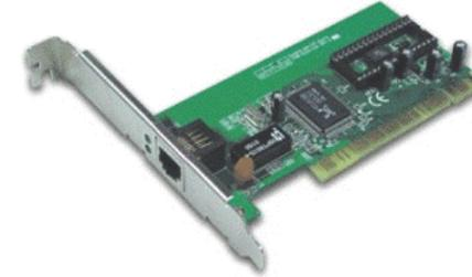
Figura 2.3 Tarjeta Ethernet
