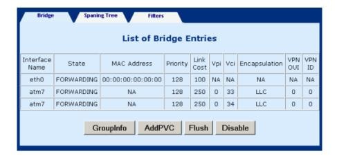
♦ **GroupInfo:** This configures the LAN packets that will travel through the LAN interface to the selected WAN interfaces. If you wish to change the interfaces that are configured you must first click on the **Flush button** (to remove the current ocnfiguration), and then click on the **Group Info** button, select the group interfaces and then click the **Apply** button. You must select eth0, as eth1 is not enabled for this product version.
