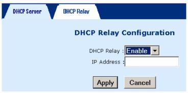
**STEP 2:** In the DHCP Relay field, select **Enable**, and enter the IP Address you want to receive BOOT REQUEST or DHCP packets from clients.
