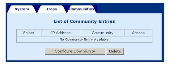
There is no community set up by factory default. To add or modify an entry, click the Configure Community button. To delete an entry, tick the entry and click the Delete button. The following screen displays after clicking the **Configure Community** button. Enter the parameters and ten click the **Apply** button.
