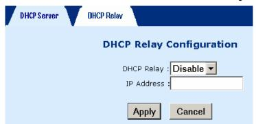
**STEP 2:** In the DHCP Relay field, select **Disable**, and enter the IP Address you want to receive BOOT REQUEST or DHCP packets from clients.
