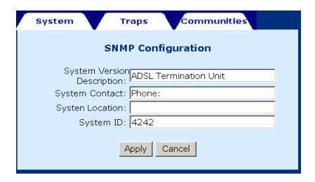
To configure the SNMP agent, click the Configure SNMP Agent button. After filling out the fields, click Apply to submit the settings.
